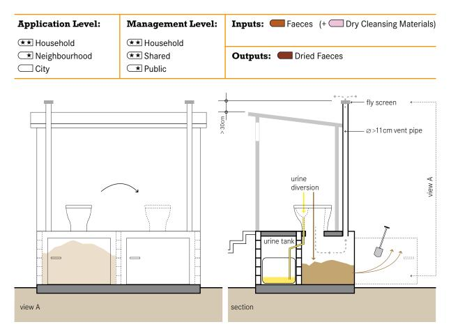
Dehydration vaults are used to collect, store and dry (dehydrate) faeces. Faeces will only dehydrate when the vaults are well ventilated, watertight to prevent external moisture from entering, and when urine and anal cleansing water are diverted away from the vaults.
